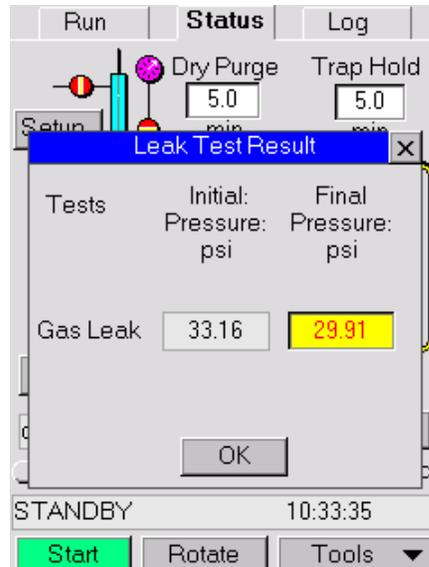
Figure 26 Failed Leak Test
