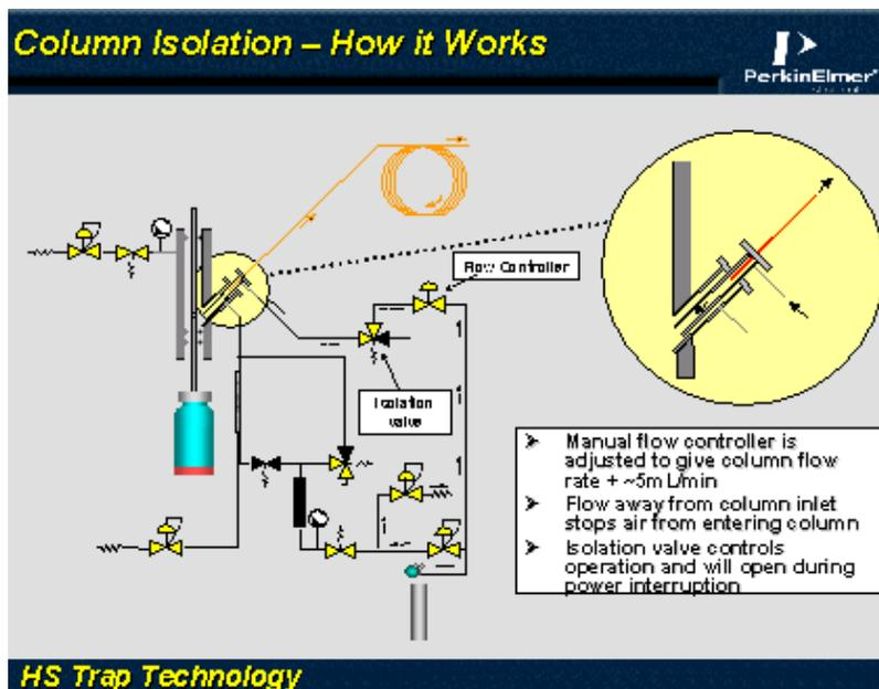
**Figure 126 Column Isolation Flow**
