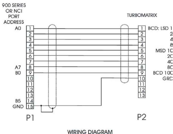
**Figure 61BCD Interface Data Channel Contacts**
