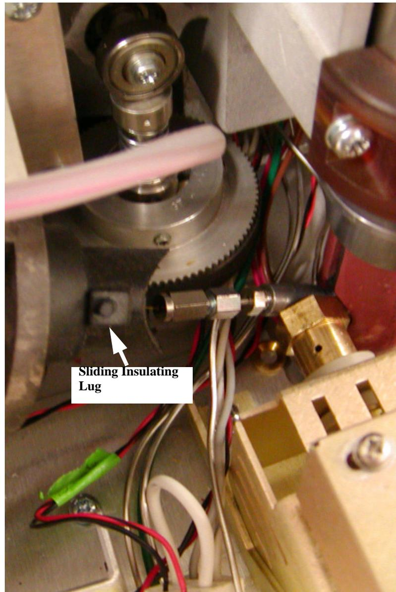
**Figure 14 Installation of Transfer Line at the Needle Unit**
