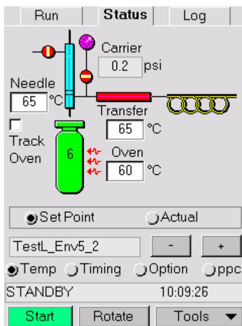
Figure 35 Temperature Tab
