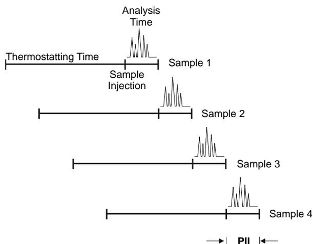
**Figure 75 Overlapping Thermostating**
