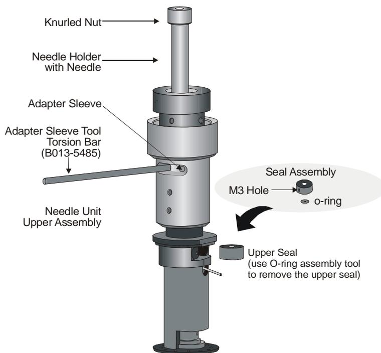
**Figure 97 Changing the Upper Seal Assembly**
