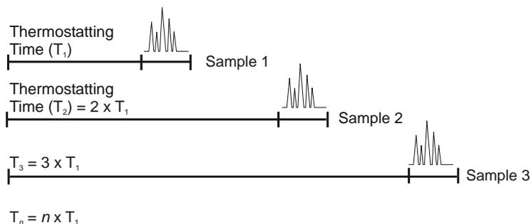
**Figure 90 Thermostating Time Using Progressive Mode**
