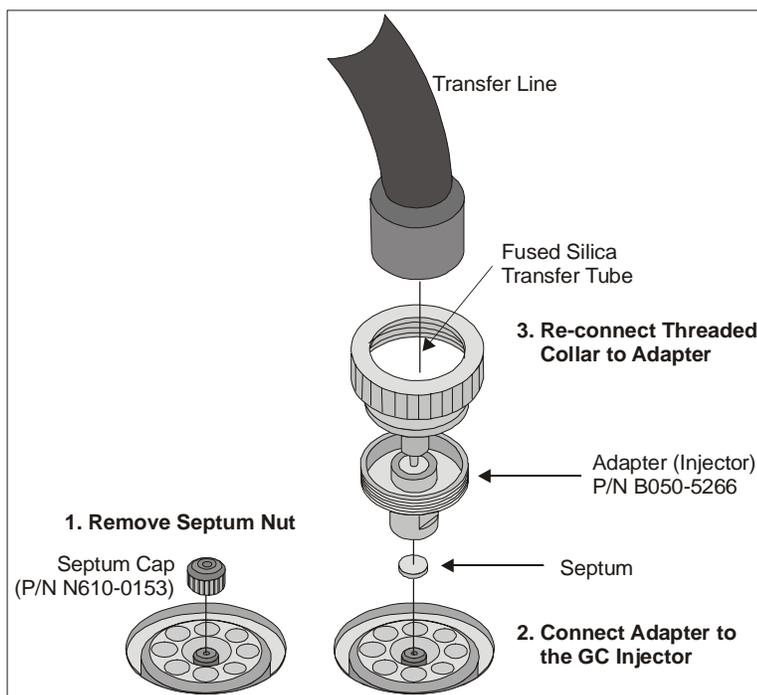
**Figure 18 Installing the Heated Transfer Line at the PerkinElmer GC Injector**
