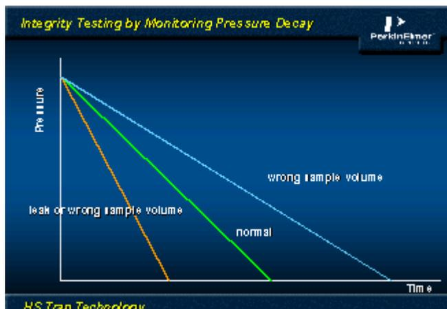
**Figure 131 Pressure Decay in Vial with a Fixed Flow Venting**
