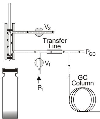
**Figure 83 High Pressure - Standby**
