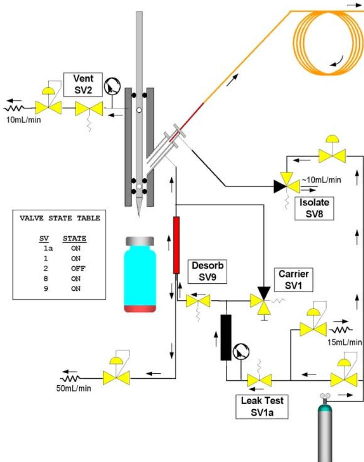
**Figure 122 Split Trap Test**
