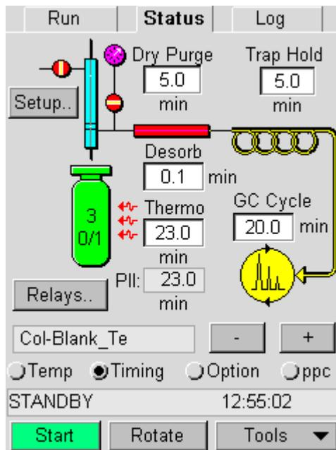
Figure 40 HS 40/110 Trap Status Tab Timing Tab
