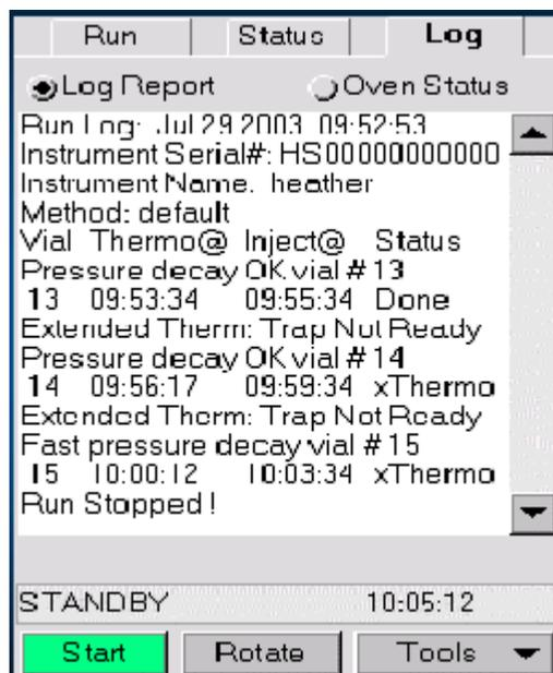
**Figure 49 Pressure Decay Log Screen**
