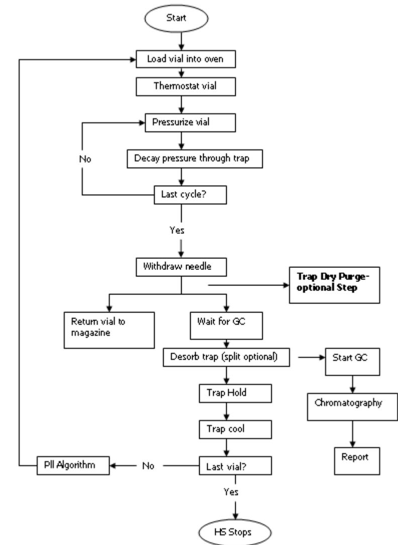
**Figure 58 HS Trap Logic flow Diagram**
