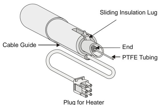
**Figure 9 The HS End of the Transfer Line**
