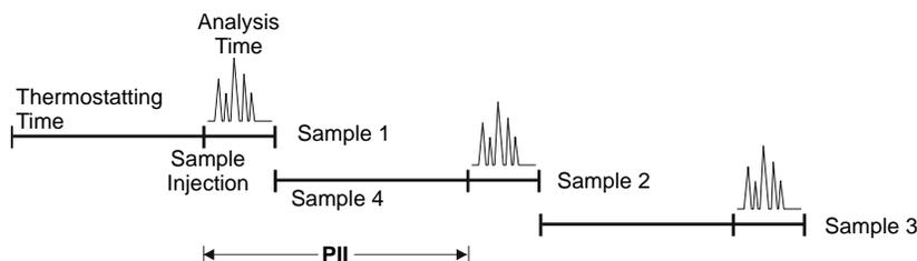
**Figure 88 Sequential Thermostating**
