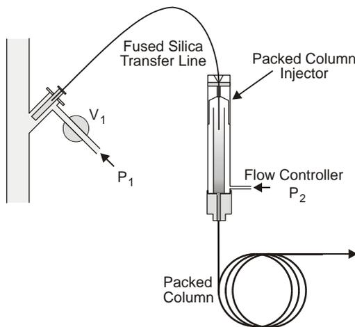
**Figure 94 Sampling with Packed Columns**
