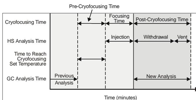
**Figure 66 Setting the Pre and Post Cryofocusing Time**
