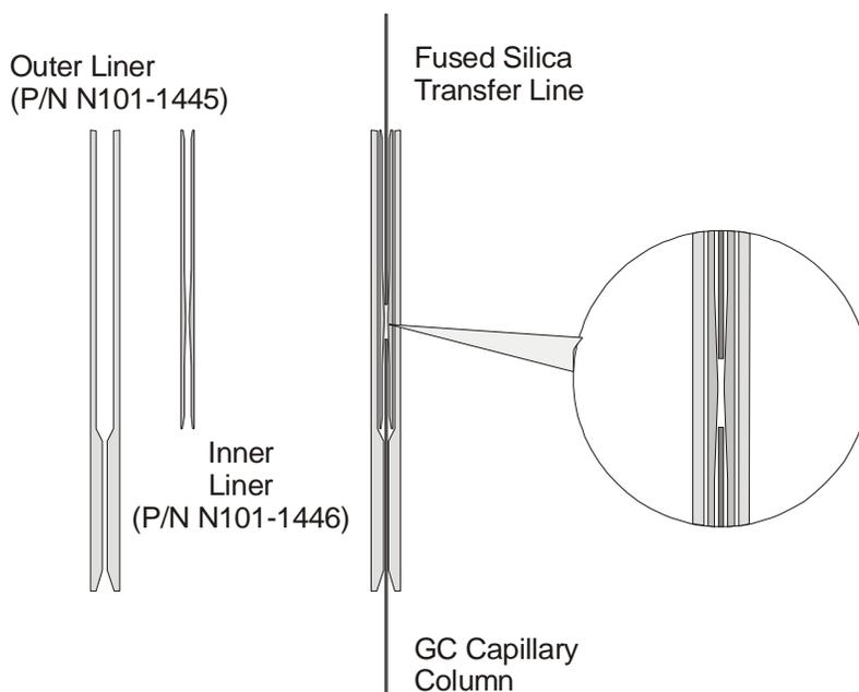
**Figure 62 Zero-Dilution Split Injector Liner**
