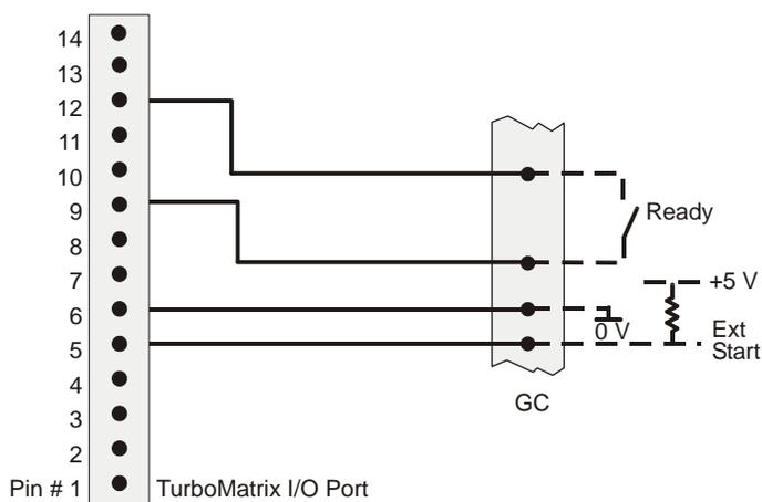
**Figure 5 Connecting the HS to Another GC Using the Ready/Start Cable**
