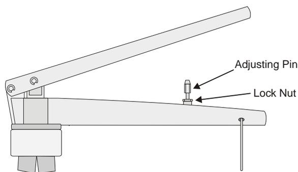
**Figure 112 Hand Crimper Locking Nut**
