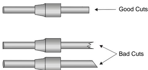
**Figure 15 Cutting the Fused Silica Transfer Line**
