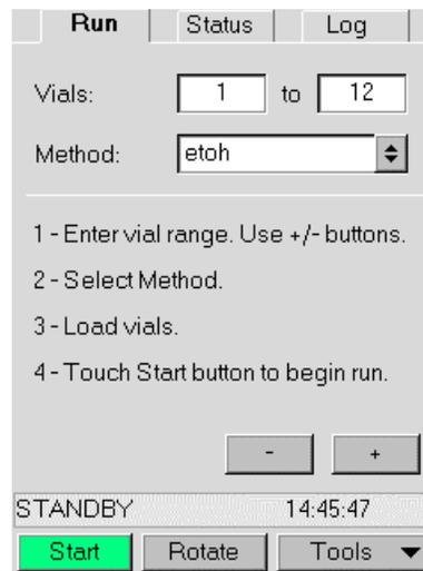
**Figure 33 Run Tab - Single Method Operation**
