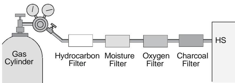
**Figure 19 Connecting Filters to the Gas Supply System**
