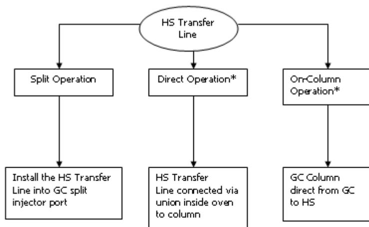
**NOTE:** If liquid autosampler is installed, the transfer line must be installed outside of the autosampler path.
