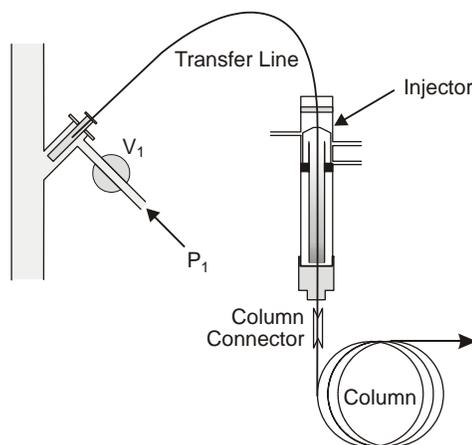
**Figure 93 Splitless Sampling – Direct Connection**
