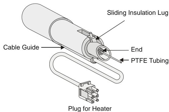
**Figure 12 The HS End of the Transfer Line**
