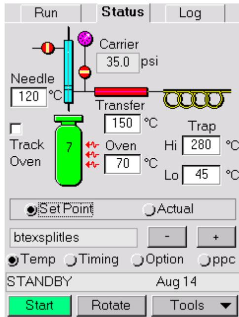
**Figure 39 HS 40/110 Trap Status Page Temp Tab**
