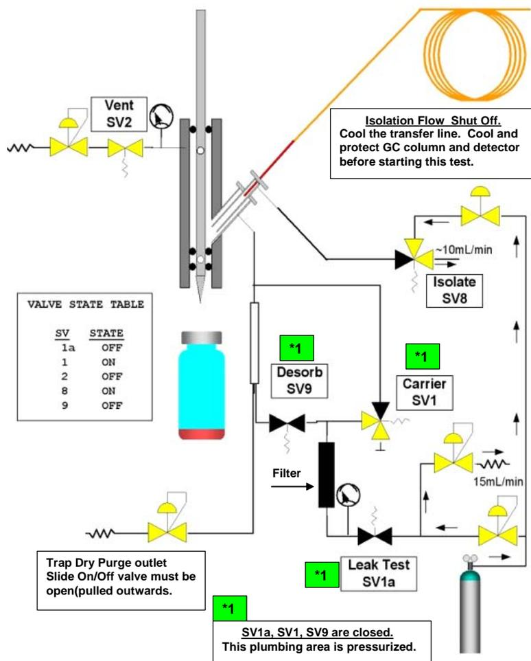
**Figure 111 Valve Leak Test**
