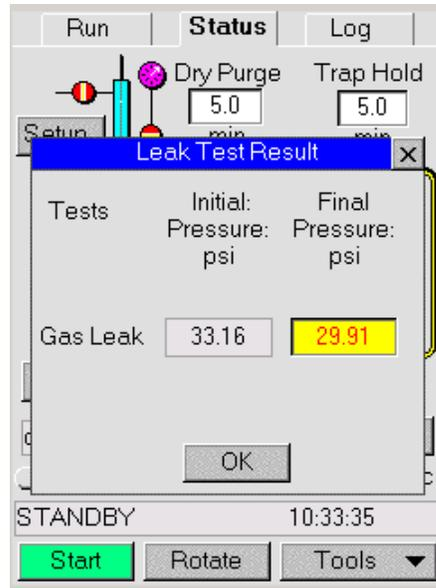
Figure 29 Failed Test (Red Text)
