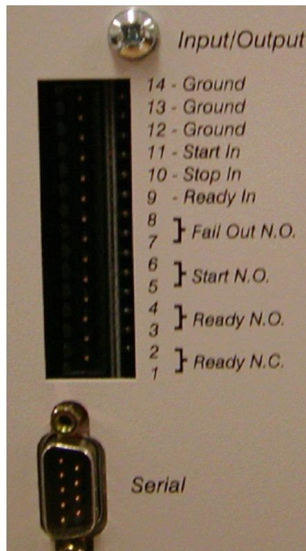
Figure 1 The HS Input/Output (I/O) Port (Diagram and Photo)
