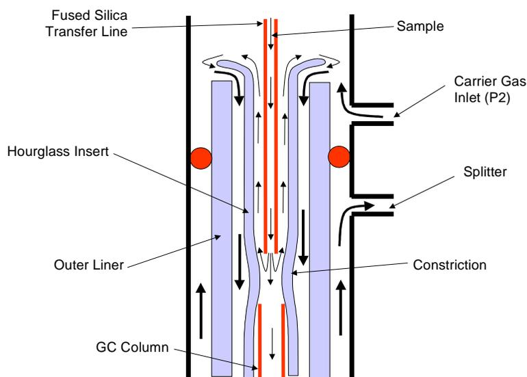
**Figure 64 Sample Flow Through the Zero Dilution Liner**
