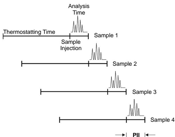
Figure 87 Overlapping Thermostating
