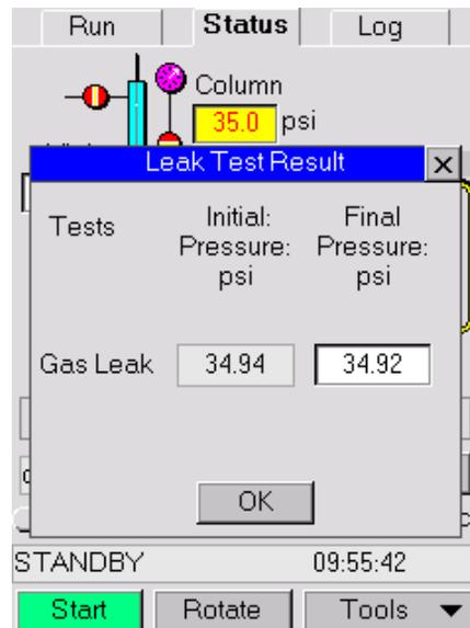
Figure 27 Passed Leak Test
