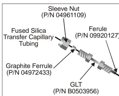
**Figure 10 Assembling the Fittings Ahead of the GLT Connector**
