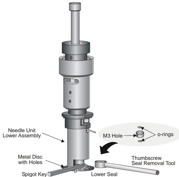
**Figure 98 Changing the Lower Seal Assembly**
