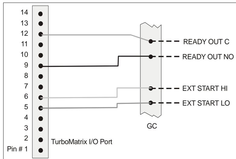
**Figure 4 Connecting the HS to the AutoSystem XL GC using the Ready/Start Cable**
