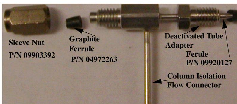
**Figure 13 Assembling the Fittings Ahead of the Deactivated Tube Adapter**
