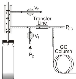
**Figure 86 High Pressure - Withdrawal**
