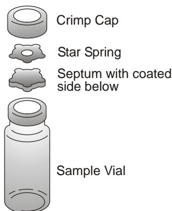
**Figure 69 Safety Closure Assembly**
