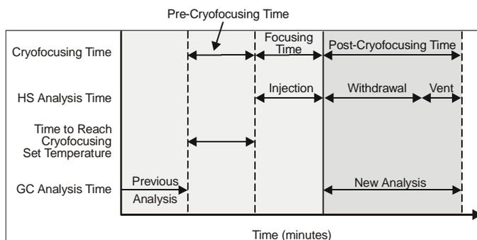
**Figure 81 Setting the Pre and Post Cryofocusing Time**
