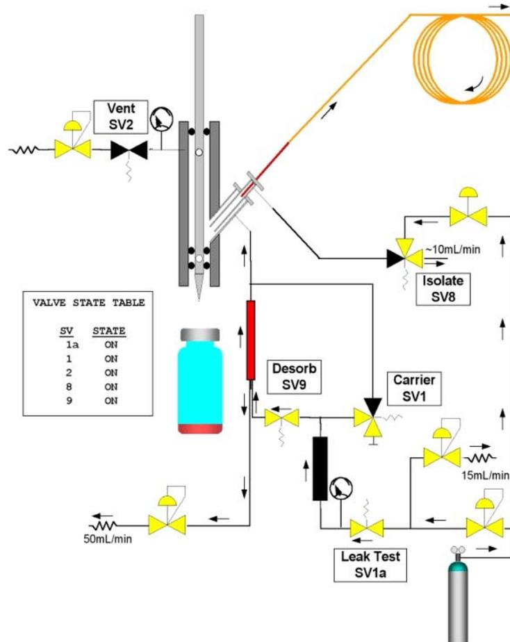
Figure 123 Splitless Trap Test
