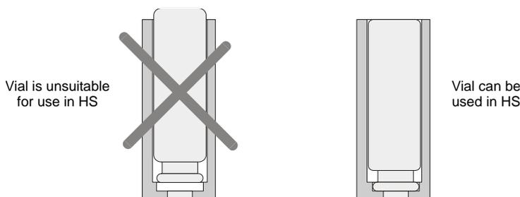
**Figure 68 Using the Vial Gauge**
