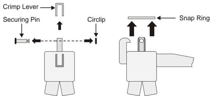
**Figure 113 Removing the Circlip and Snap Ring**
