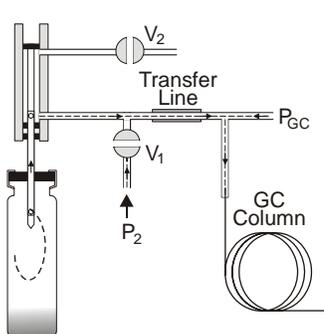
**Figure 85 High Pressure - Sampling**
