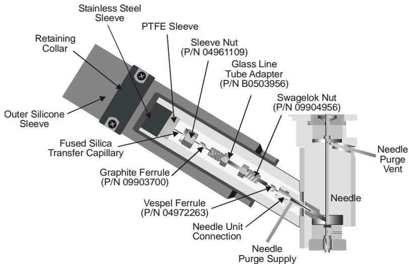
**Figure 11 Installation of Transfer Line at the Needle Unit**
