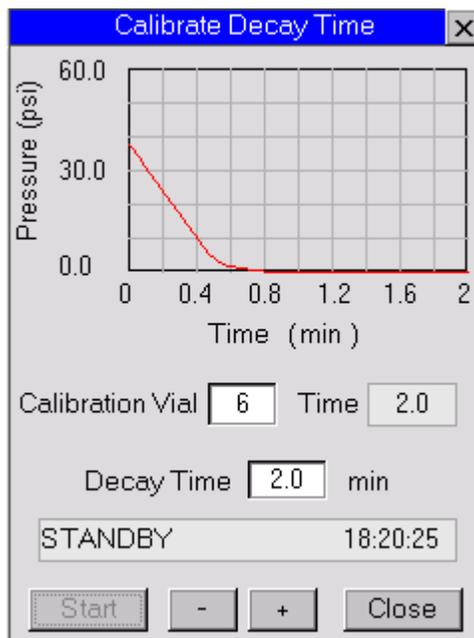
**Figure 44 Example of Fast Pressure Decay Curve**
