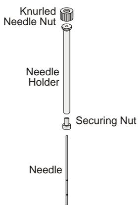
**Figure 96 Changing the Sampling Needle**
