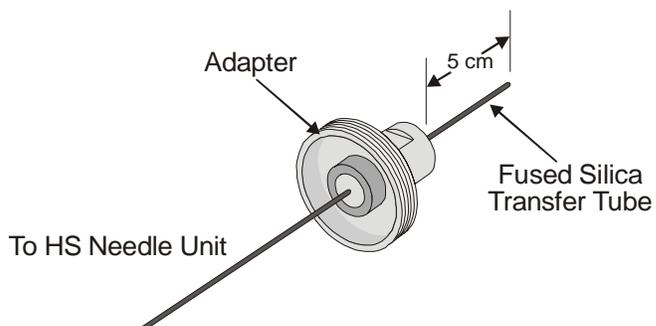
**Figure 17 Length of Transfer Line that Must Extend Past the Adapter for Installation at GC**
