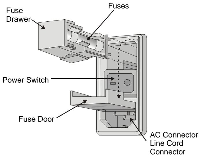
**Figure 95 Replacing the Fuse**
