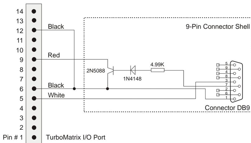
Figure 6 Schematic of the HP Sampler Cable
