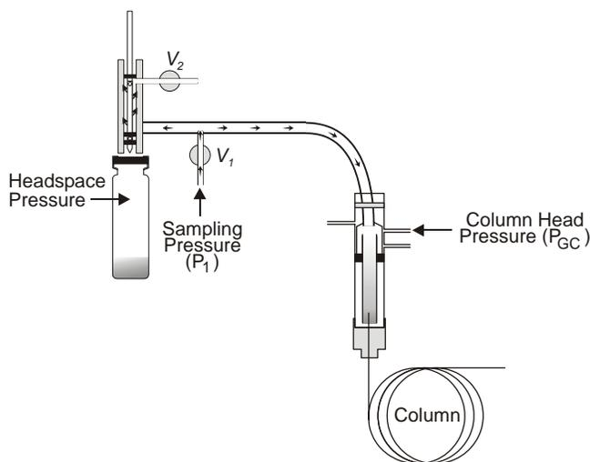
**Figure 92 System Pressure During Split Operation**
