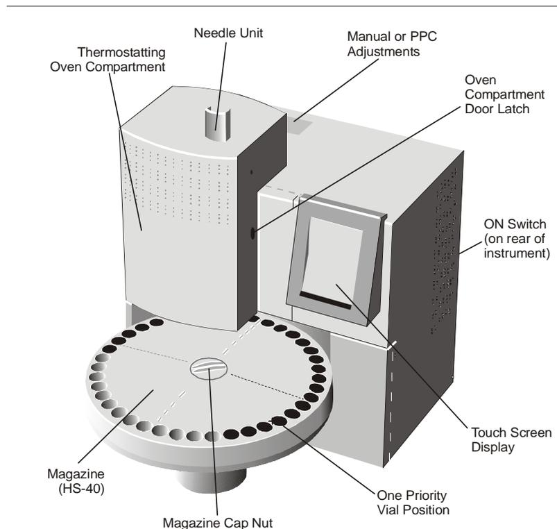
**Figure 32 Layout of the TurboMatrix Headspace Sampler**
