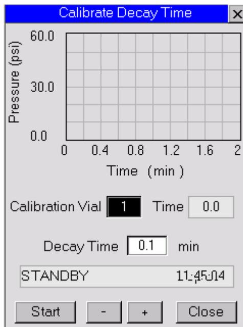
**Figure 42 HS 40/110 Trap Calibrate Decay Time Screen**
