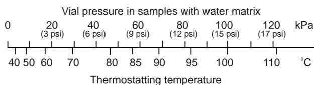
**Figure 74 Relationship Between Vial Pressure and Thermostating Temperature in Samples with a Water Matrix**
