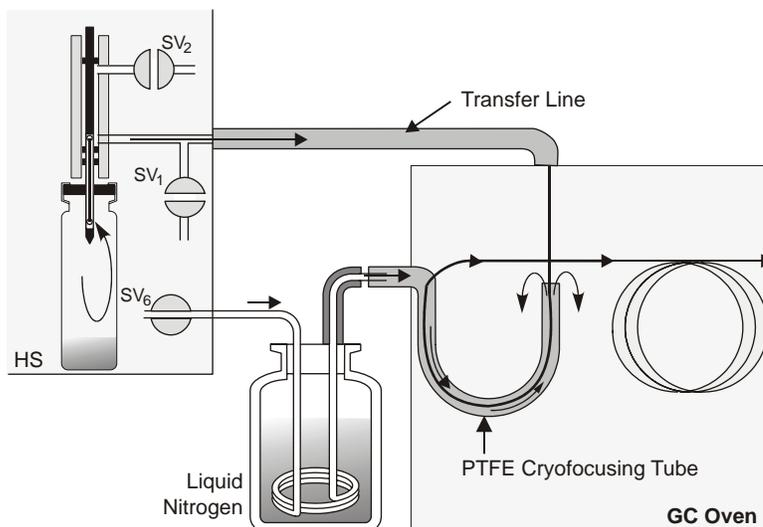
**Figure 65 Cryofocusing Accessory**
