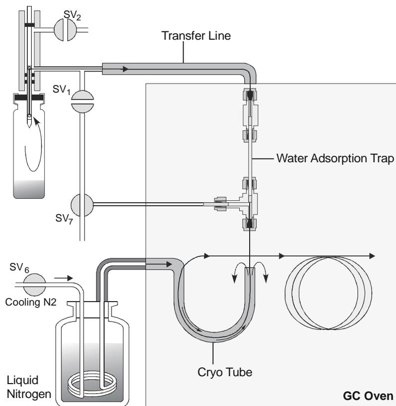
**Figure 67 Cryofocusing with the Water Adsorption Trap**
