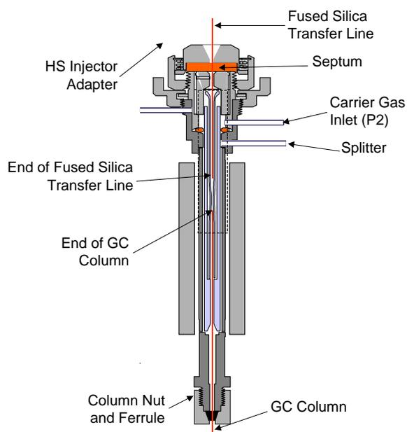
**Figure 63 Cross Section of the Zero-Dilution Split Injector Liner Installed in the GC Injector**
