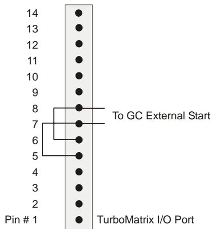
**Figure 2 Connecting the Fail Output Signal in Parallel with the Start Signal**
