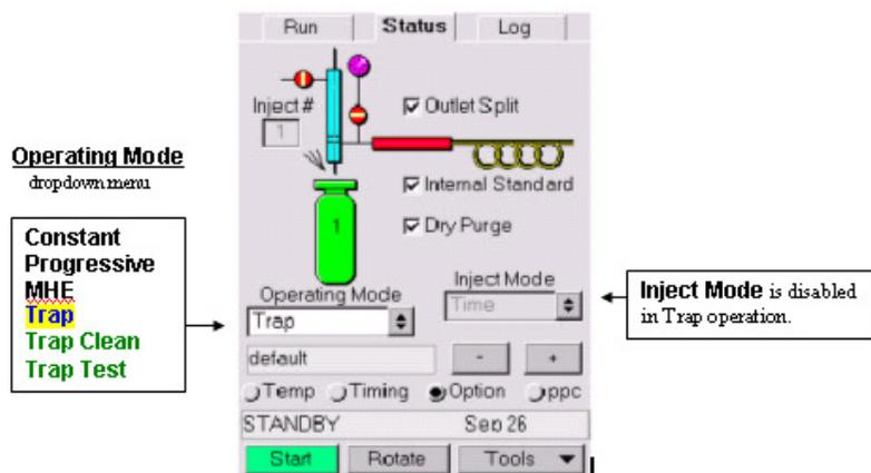
Figure 45 HS 40/110 Trap Status Tab Option Tab
